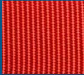
1001 NYLON Commercial Type 10 1.75" wide | Tensile 9500#
